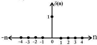
In words the unit sample sequence is a signal which give only u nit value at n = 0 and Zero value except  $n \neq 0$ .
