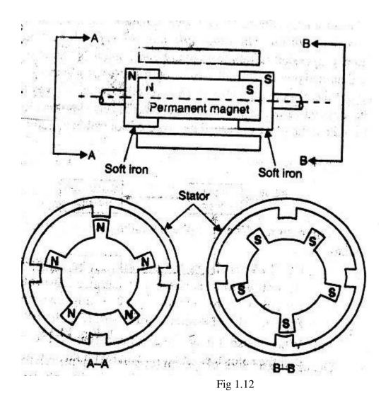
The rotor teeth are machined on the sot iron stacks. Thus the rotor teeth on one end become the north pole and those at the other end become the south pole.
