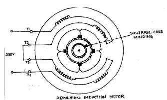
i) The stator carries a single distributed winding fed from single-phase supply. ii) The rotor is provided with two independent windings placed one side the other. The inner winding is a squirrel-cage winding with rotor bars permanently short circuited. The outer winding is a repulsion commutator armature winding placed over the squirrel cage winding.
