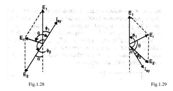
Since,  $R_a$  is very small as compared to  $X_s$ ,  $\theta$  is nearly  $90^o$  so that the current  $I_{sy}$  is almost in phase with  $E_1$  & in phase opposition to  $E_2$ . This means that machine 1 is generating and machine 2 is motoring. consequently, the machine 1 tends to slow down and machine 2, by accepting power, tends to accelerate. This restores the status quo i.e., synchronism is re established.
