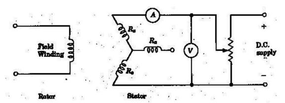
Fig.1.10 D.C. resistance test on an alternator.
