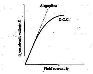
Fig.1.12 The O.C.C. of an alternator
