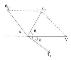
If the motor is further loaded, its rotor further back by a greater value of load angle ' ' the resultant voltage 'ER' is increased and the motor draws an increased armature current but at a devised power factor.
