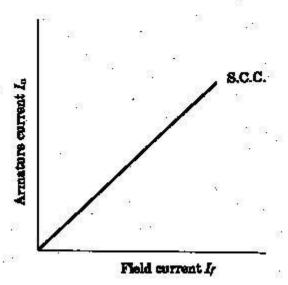
Fig.1.14.The S.C.C of an alternator
