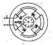
Figure 5 shaded pole motor
