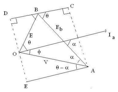
Mechanical power per phase developed in the rotor is  $P_m=E_bI$  cos
