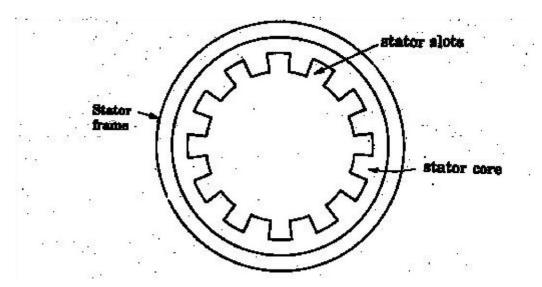
Figure 1.1 Alternator stator
