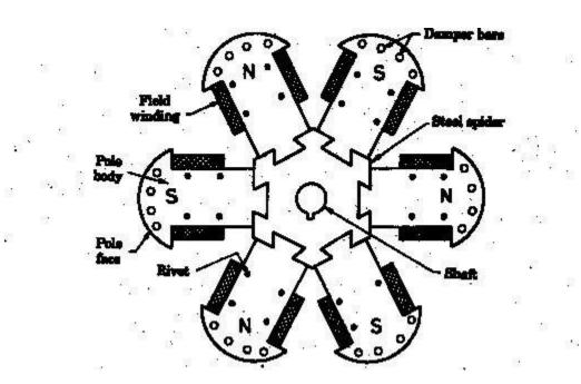
Figure 1.2 Six-pole salient-pole rotor
