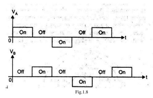
(iv) So far the rotor has completed one-half revolution. However, if we continue the appropriate switching the rotor will complete one revolution in 90° steps.
