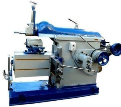
Hydraulic Type Shaper Machine
