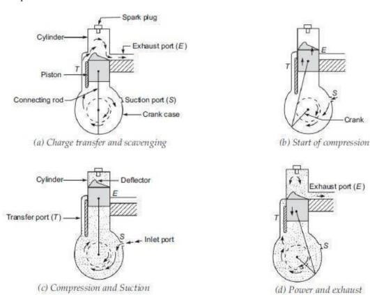
The following operation takes place in a two stroke or in one revolution of the engine
