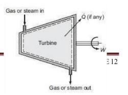
For a turbine, if it is insulated and the flow velocities are small, the kinetic terms can be neglected. Hence the SFEE is,
