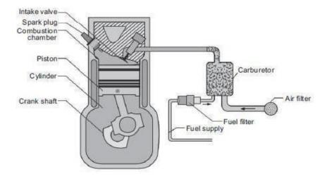
All operations are carried out in four strokes the piston, i.e., two revolutions of the crank Therefore, the engine is called a four stroke engine.
