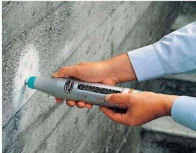
NDT test on concrete
